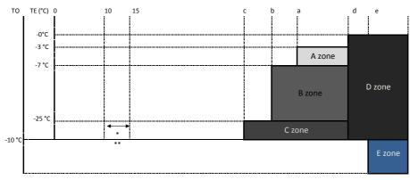
\* The minimum TE value and TO value between 10 and 15 minutes after heating operation has started are stored in memory as TE0 and TO0, respectively.
