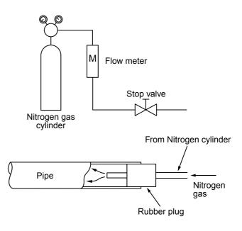
Fig. 3-5-1 Prevention of oxidation during brazing
