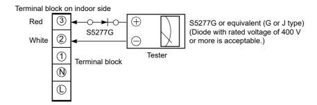
Normal time : Voltage swings between DC15 and 60V. .....Inverter Assembly check (11-7-1.)
