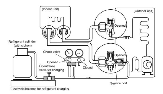
Fig. 3-4-1 Configuration of refrigerant charging
