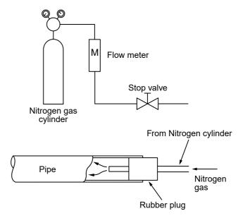
Fig. 3-5-1 Prevention of oxidation during brazing
