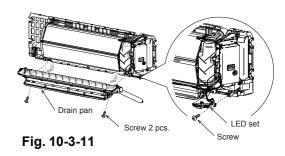
The drain hose can be removed by removing the screw securing the drain hose then secure rotate steel plate of drain hose to out of the Drain pan and pulling out the drain hose.
