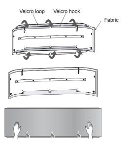
5. Reassembly the air inlet grille by reverse process of 1.
