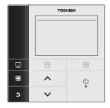
2 Press the [ ] / [ ] button to select "FC for Hydro unit" on the FIELD SETTING screen, then press the [ ] button.
