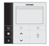
Press the [ ]/[ ] button to select "Test mode" on the FIELD SETTING MENU screen, then press the [ ] button.
