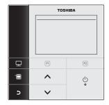
2 Press the [ ] / [ ] button to select "FC for Hydro unit" on the FIELD SETTING screen, then press the [ ] button.
