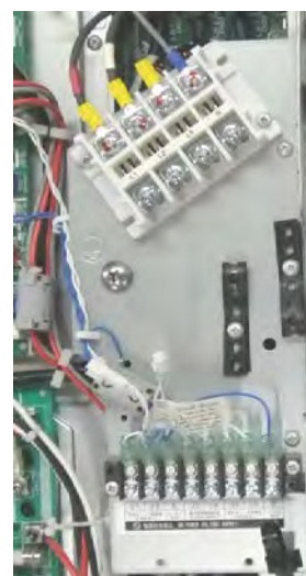
close-up view of terminal block sub-assembly
