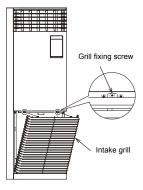
The intake grille is fixed by the screws for safety reasons. Use a screwdriver to unfasten the screws of the intake grille (two places) to open the intake grille. The screws are designed to stay on the intake grille.
