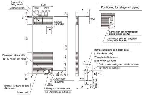
\* Drain hose drawing-out port (Both side) is for only RM110 model to RM160. To connect drain hose on right or left, route it through the knock-out for refrigerant piping on RM56 to RM80 model.
