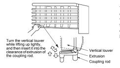
The direction of the auto turn louver (Vertical louver) may change during transportation. As shown below, lift up the vertical louver lightly, turn it matching with the direction of the plastic coupling rod, insert it into clearance of the extrusion, and then arrange the direction of the vertical louver to the desired direction.
