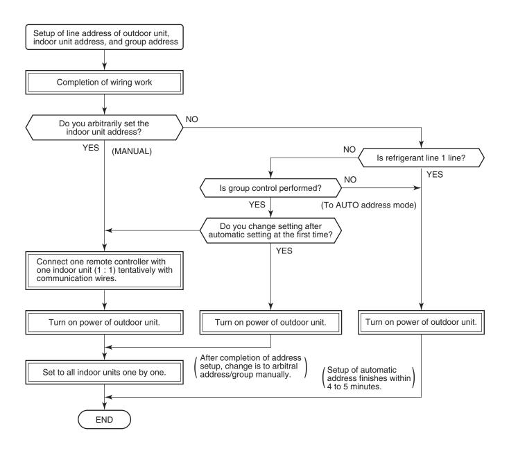
When the following addresses are not stored in the EEPROM on the indoor P.C. board, a test run operation cannot be performed. (Unfixed data at shipment from factory)
