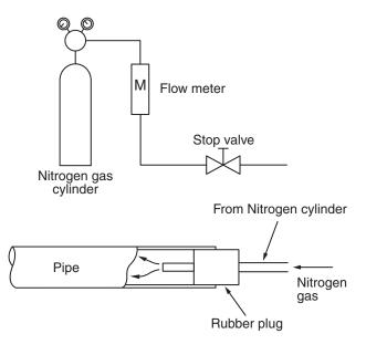
Fig. 6-5-1 Prevention of oxidation during brazing
