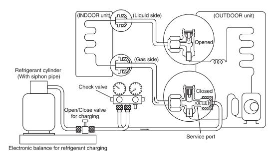
Fig. 6-4-1 Configuration of refrigerant charging
