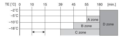
\* The minimum TE value during 10 and 15 minutes after starting heating operation is stored as TEO.
