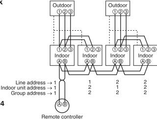
(Example of 2-lines wiring) (Real line: Wiring, Broken line: Refrigerant pipe)
