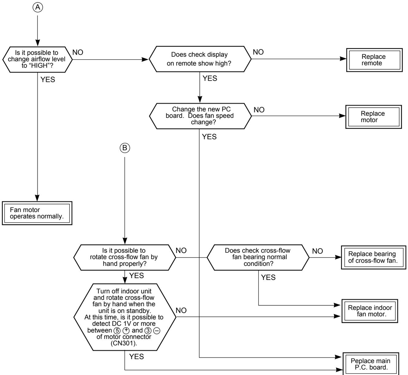
**(4) Indoor fan motor automatically starts to rotate by turning on power supply**
