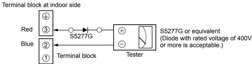
Normal time : Voltage swings between DC15 and 60V. .... Inverter Assembly check (11-8-1.)
