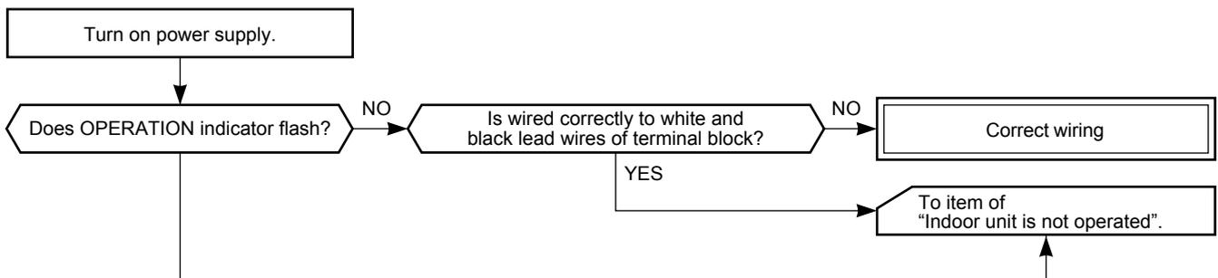
**(3) Only the indoor motor fan does not operate**
