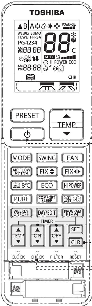
**1** Press [CHECK] button with a tip of pencil to set the remote controller to the service mode.
